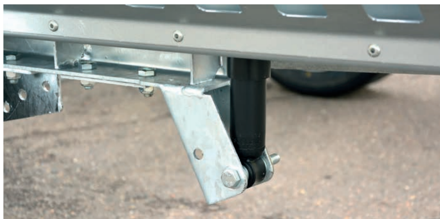
Dumping body can be tilted with dampers (maintenance free, hydraulic)
