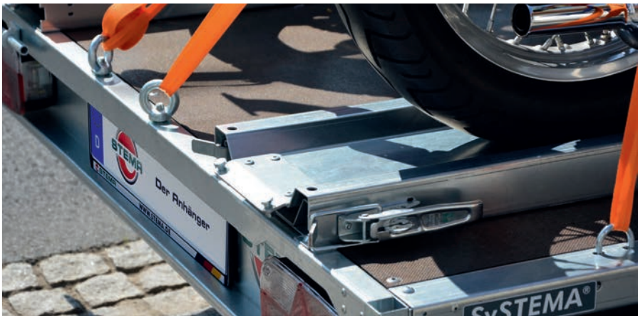
the STLP 850 has 4 additional retractable lashing eyes
