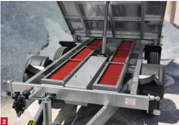
galvanized steel base with eight retractable heavy duty lashing rings
